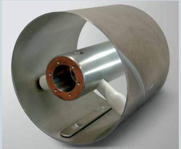
Cross-section through a GIL of the 2nd generation showing conductor tube, enclosure, paired post insulators and integrated particle trap
